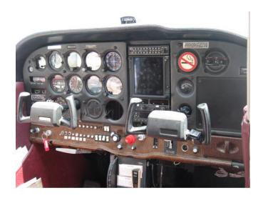
(PIC 1) Typical analog instrument panel from the early 1980s, (with one modern radio). This is a 1981 Cessna 172; the airplane I often instruct in came along, and then were sufficiently mass-produced that the cost came down, that computer screens made their way into small airplanes.
